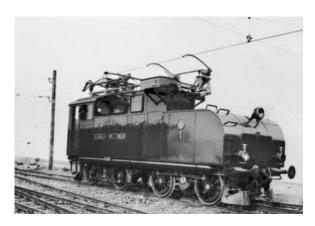
The experimental locomotive no. 1 with rotary converter and DC traction motors made by Maschinenfabrik Oerlikon AG which was aquired by BBC and merged to ABB.
